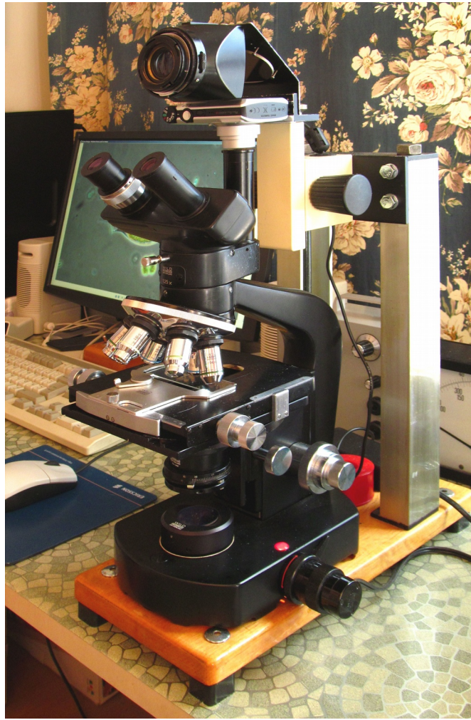
Wild M 20 with rotatable stage, Canon A3200 camera and camera mirror and focusing lens. (2015).
