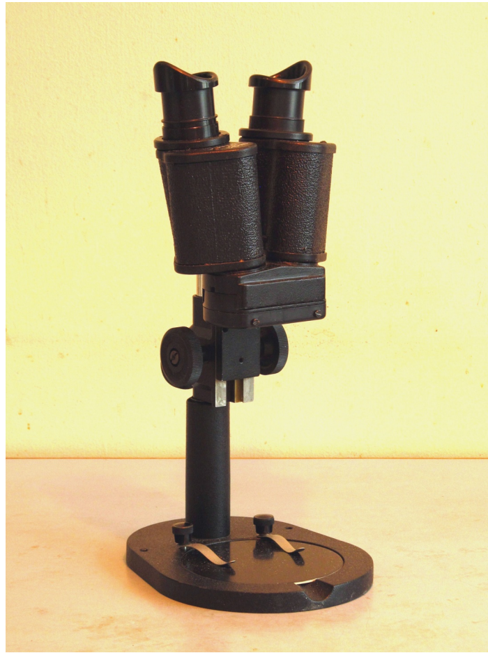
The fixed 8,75x stereo microscope BM-51-2 (1998).
